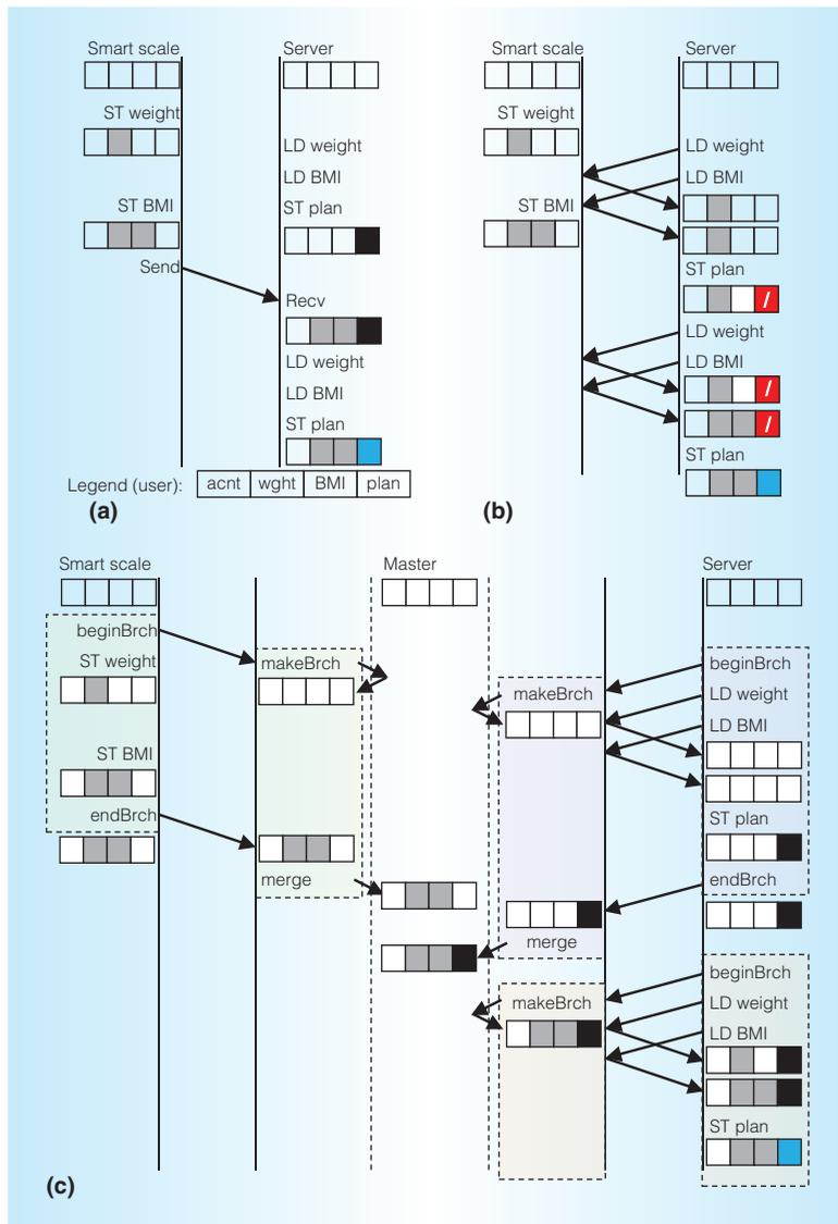
Figure 3. Timing graphs of communicating shared data. (a) Message passing; (b) IoT-HDSM without branch; (c) IoT-HDSM with branch. Without the memory branch annotation, the server could read a partly updated set of data, such as gray weight and white BMI variables. The branch annotation allows the smartphone and the server to operate on a snapshot of a shared memory.
