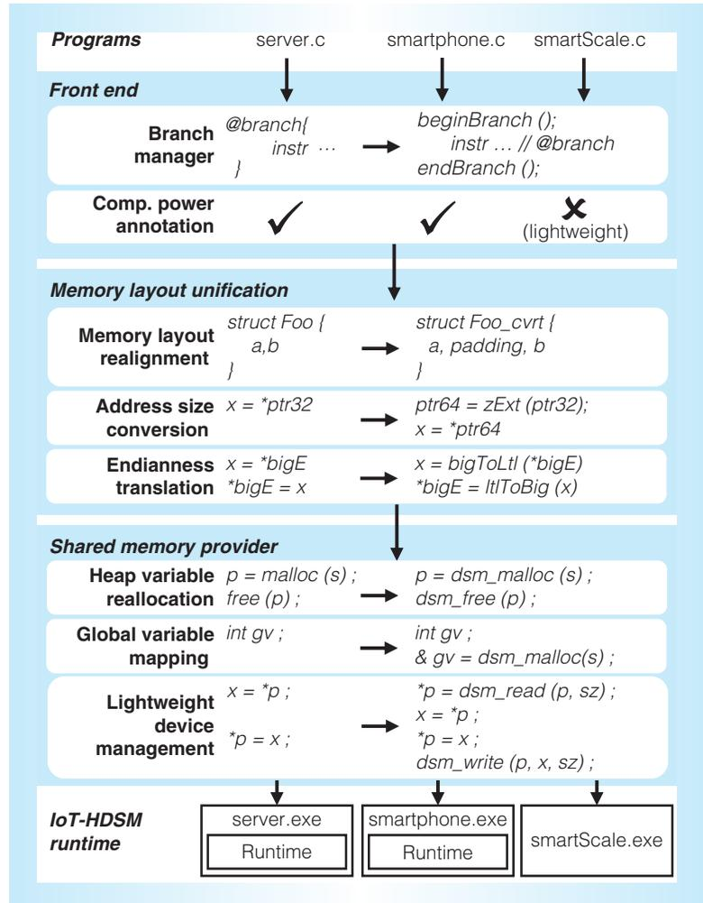
Figure 4. Overall structure of IoT-HDSM framework with the programs in Figure 2. The IoT-HDSM compiler modifies data structures and inserts translation instructions to integrate heterogeneous memory layouts. The compiler inserts explicit communication codes for shared data accesses to support lightweight devices that cannot execute the IoT-HDSM runtime.
