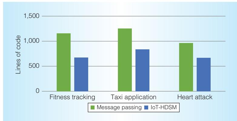
Figure 6. Lines of code (LoC) of IoT applications. IoT-HDSM simplifies the IoT programming by requiring 35.56 percent fewer lines of code than the message passing model.
