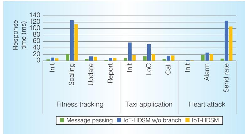
Figure 5. Response time for each event in IoT applications. Compared to the message passing model, the IoT-HDSM framework suffers from 24 ms and 100 ms average and maximum latency overheads. The memory branch annotation yields the geomean speedup of 1.33 times beside the non-branch version.
