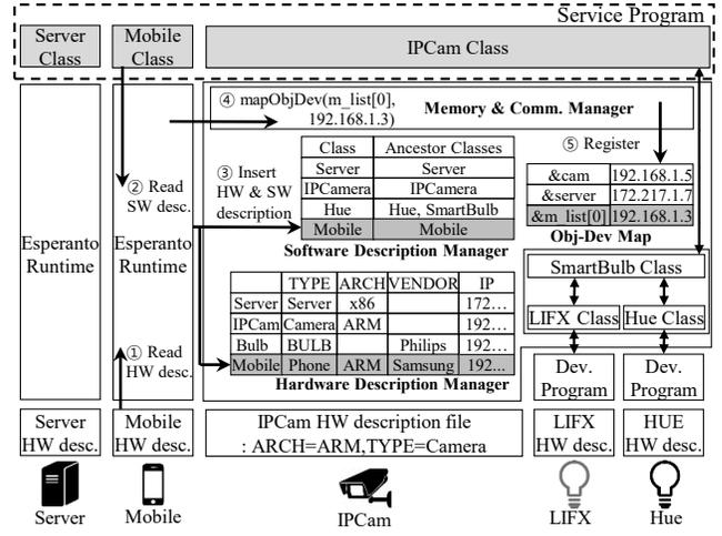
Figure 8. The overall structure of the Esperanto runtime
