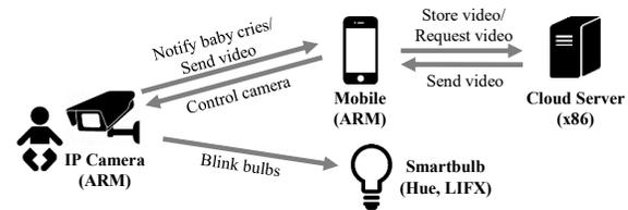
Figure 1. An IoT service example: Baby monitor
