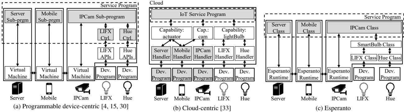
**Figure 2.** The overall structures of the baby monitor program (Figure 1) in different IoT frameworks. Here, the baby monitor program executes customized sub-programs for multiple programmable devices such as the IP camera, the server and the mobile, exploiting third-party devices such as Hue and LIFX smartbulbs. Gray boxes are programs that programmers need to write, and dashed boxes are integrated programming views that each framework provides.
