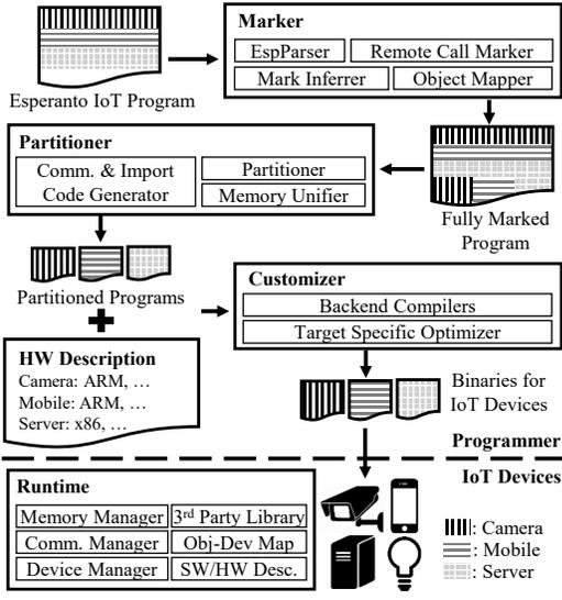
Figure 5. The overall structure of the Esperanto compiler
