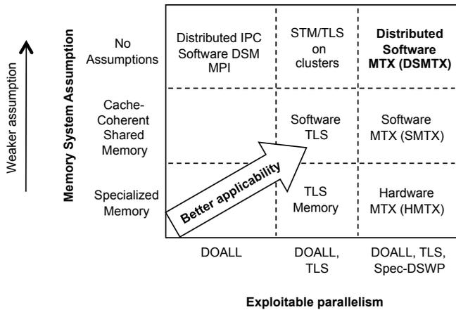
Figure 2: DSMTX enables the widest variety of parallelization paradigms, while making the fewest assumptions about the underlying hardware.
