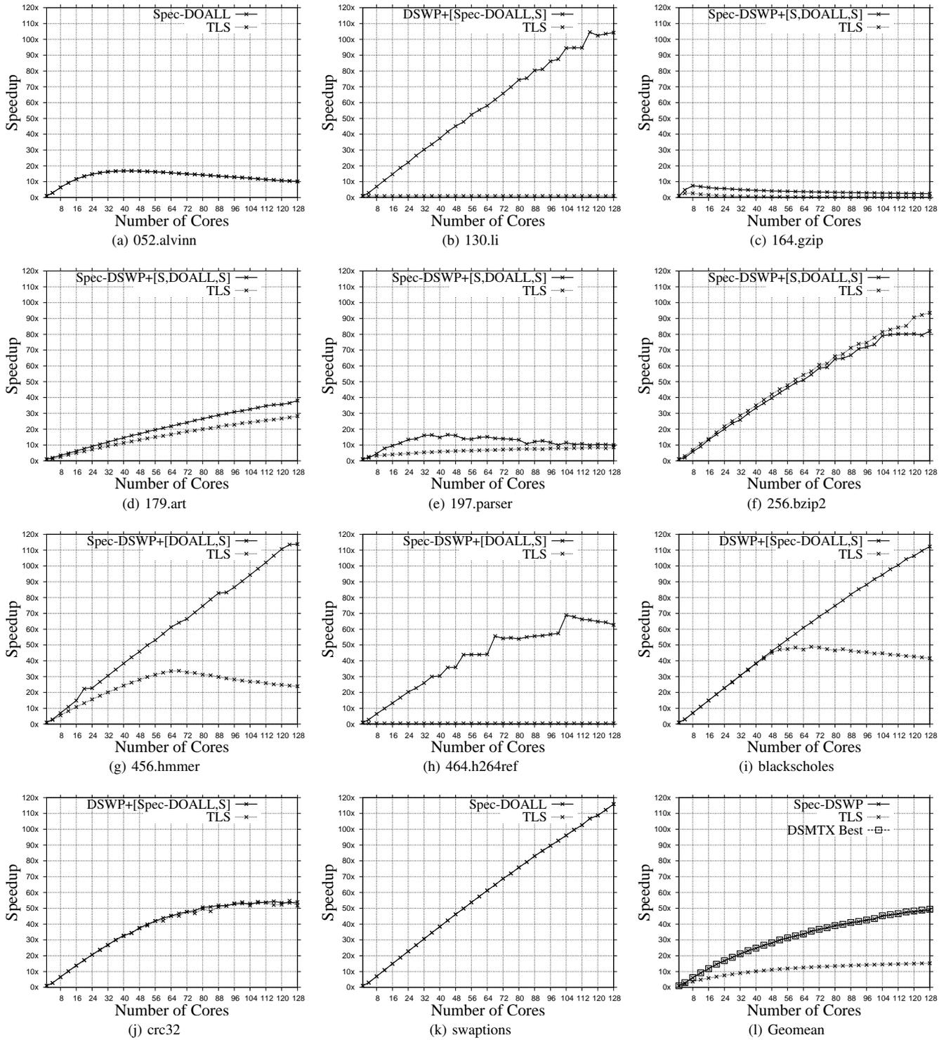
Figure 4: Performance scalability of Spec-DSWP and TLS using DSMTX
